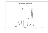
Identifying elemental compounds with the Spherical Grating Monochromator. We found very specific signatures for Calcium. Our samples (left) match the spectrum for calcium carbonate ( $\text{CaCO}_3$ ) as illustrated on the right from Nafie et al. 2001.
